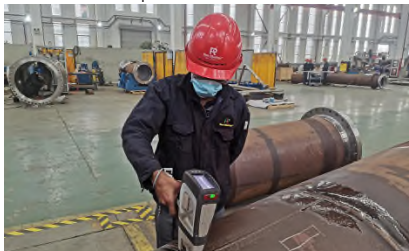
Weld Joint PMI
