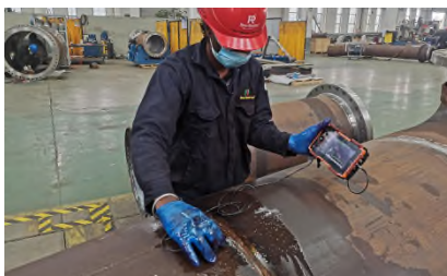
Weld Joint UT
